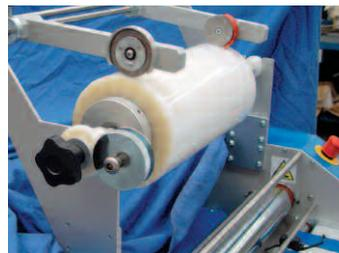
A film splitter is provided to allow non-standard sheet sizes to be run when using a wider standard width film, reducing the need to carry stocks of non-standard film widths.
