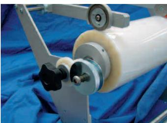
The film mandrel is capable of accepting both 25mm and 76mm core sizes.
