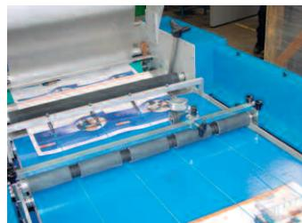
The automatic sheet separator is adjustable to separate any size of sheet up to B2 and allows the laminator to be run by a single operator.
