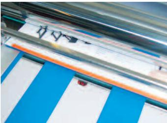
A 'missing sheet' detector stops the laminator if no sheet is detected helping to avoid messy wraparounds.
